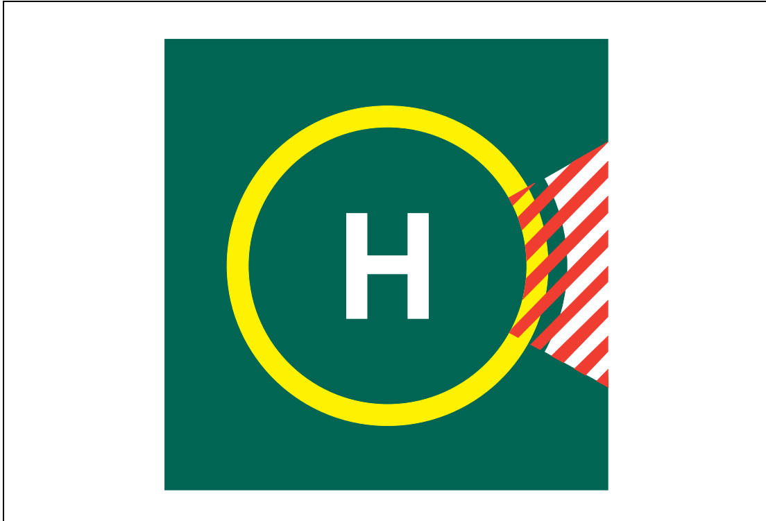
Figure 4.6 Example of Prohibited Landing Heading Marking
